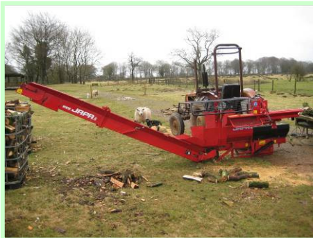
Automatic log splitting machine. This cost around £5000 and requires a 35 horse power tractor to run.
