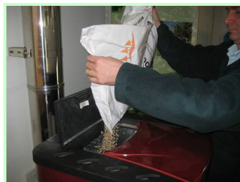
Adding wood pellets to the integral hopper. This needs to be done 1-2 times per day.
