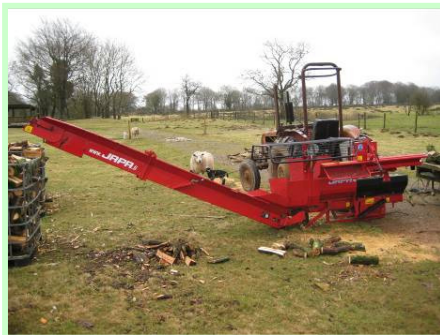
Automatic log splitting machine. This cost around £5000 and requires a 35 horse power tractor to run.
