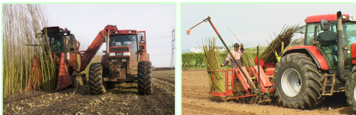
Austoft harvester and 4-row step planter in operation. (Images courtesy of Strawson's Energy, Northern Bioenergy)
