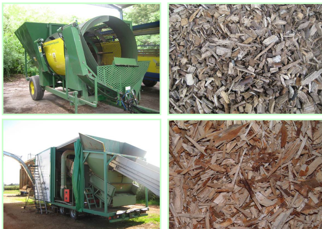
Premium quality woodfuel can be produced from SRC with mobile units.
