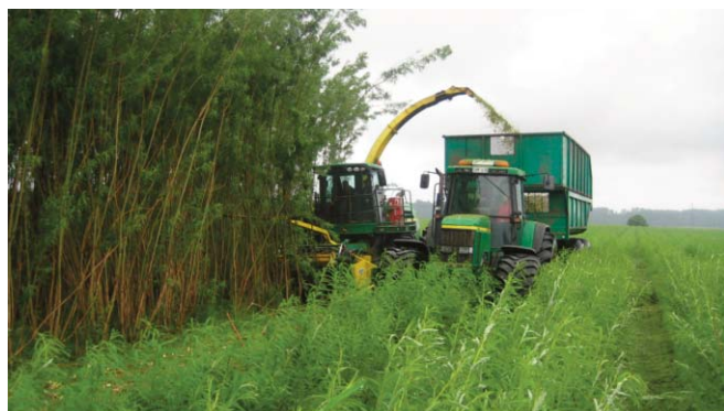
Direct chipping of willow with a JD forage harvester with a HSAB head (June 2013)
