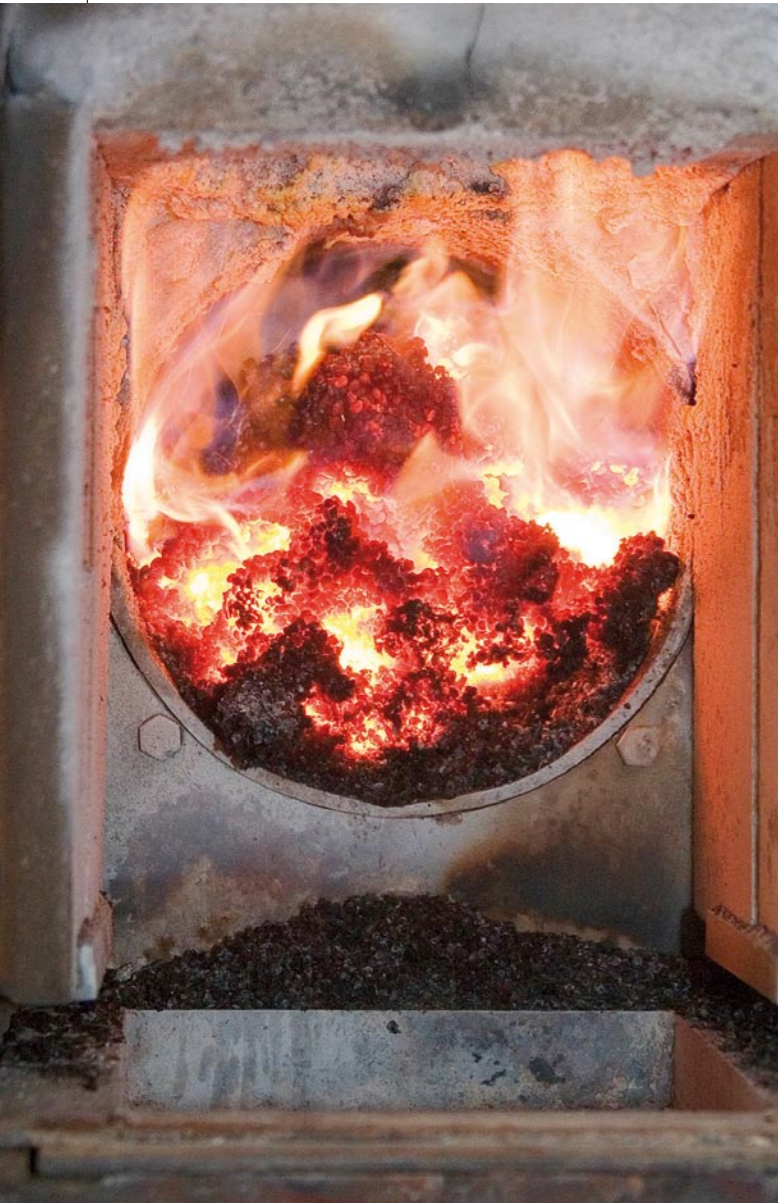
Farm 2000 biomass burner running on wheat.
