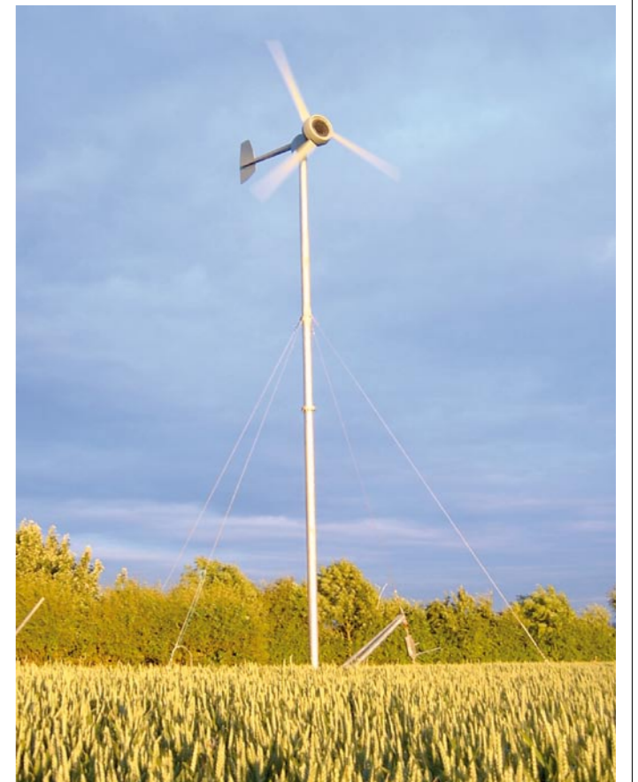
IskraWind ( www.iskrawind.com ) 5kW turbine can produce 7500kWh/year.
