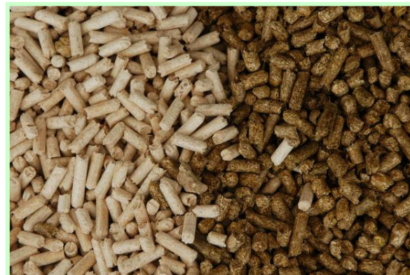
Wood pellets. The ones on the left are made of compressed sawdust whilst the ones on the right are oilseed rape meal.
