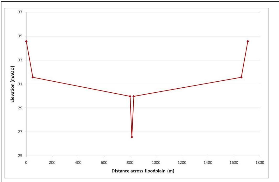
The modelled floodplain area was 5.3km<sup>2</sup>, 2.3km<sup>2</sup> of which were inundated during the simulations. The peak flow of the inflow hydrograph was 409.8m<sup>3</sup>/s. The baseline model was set up with 4m model domain resolution. As with the previous models, a 10m buffer strip of grass along the river banks was included. The coupled 1D – 2D model run time was 8 hours.
